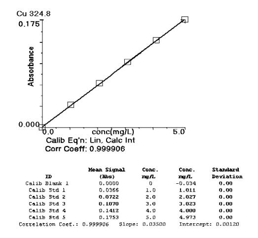
Figure 2. Calibration curve for Cu<sup>+2</sup> standarts in concentration ranges of 1-5 mg/L.
