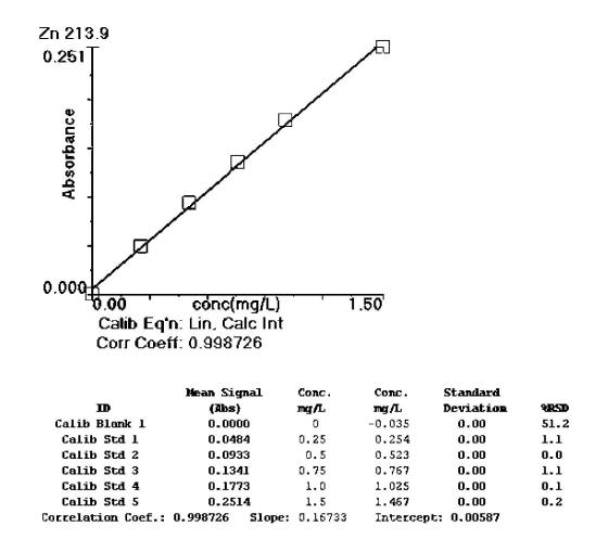
Figure 1. Calibration curve for  $Zn^{+2}$  standarts in concentration ranges of 0.25-1.5 mg/L.
