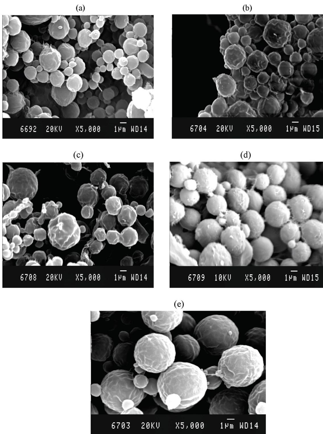
**Figure 1.** Micrographs of microparticles prepared at different stirring rates and drug:polymer ratios (a) 8000 rpm, 1:25 ratio (A10) (b) 9500 rpm, 1:25 ratio (B10) (c) 13500 rpm, 1:25 ratio (C10) (d) 13500 rpm, 6:25 ratio (C60) (e) 8000 rpm, 6:25 ratio (A60).
