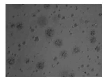
Figure 3. Microscopic view of multiple emulsion formulation F4 after preparation.
